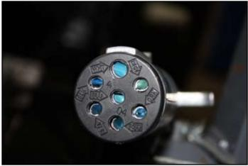
Figure 7. The 7-pin connector
