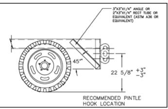
Figure 15. Use angle iron for additional support
