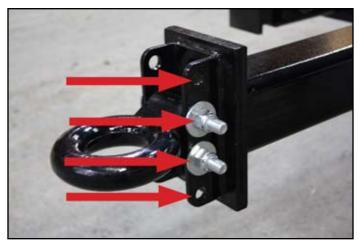
Figure 16. Adjust the receiver ring
