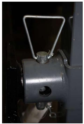
Figure 19. The jack pin is engaged
