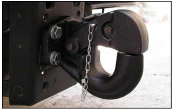
Figure 8. Use a correctly rated pintle hook
