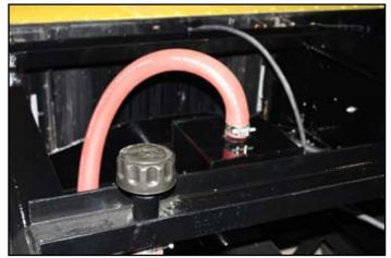
Figure 21. Check hydraulic fluid
