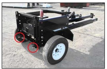
Figure 13. Loosen the jam nuts
