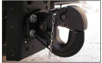
Figure 25. Check for correctly rated pintle hook
