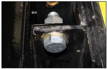
Figure 22. Check torque on mounting nuts
