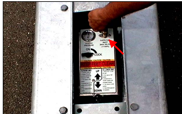
Figure 5. Connect the air supply hose to the Supply Air Inlet fitting located on the top (or on some models the end) of the Control Panel. Adjust the Supply Air Inlet regulator until you see approximately 120 psi on the System Pressure gauge.
