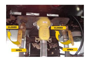
The valves are at the back of the caboose as shown in the accompanying picture. Close valves by rotating the two yellow handles as shown. CAUTION: When the brake valves are closed per the instructions above, the trailers brakes will not be on. Exercise caution and set trailer jacks as provided below to stabilize and secure.
