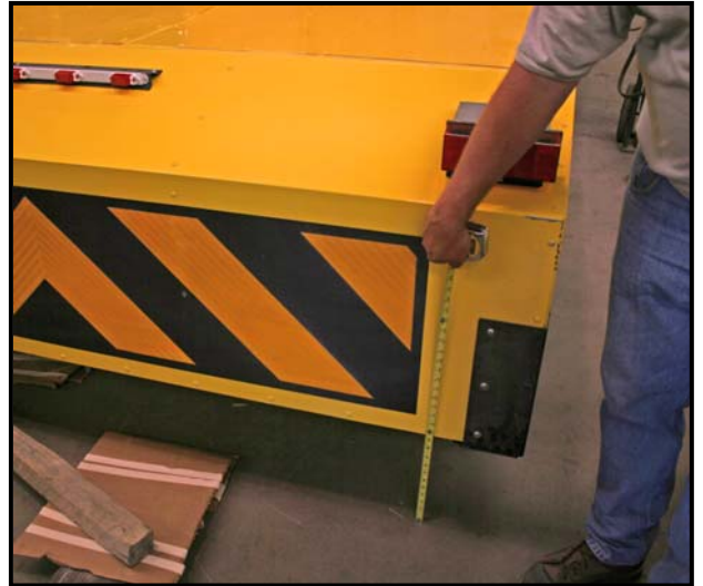
Figure 15. Adjust the level of the cartridge.
