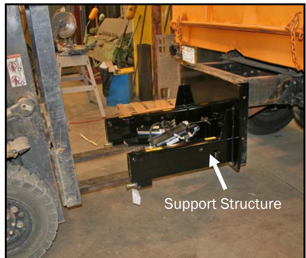
Figure 3. Fit the support structure.
