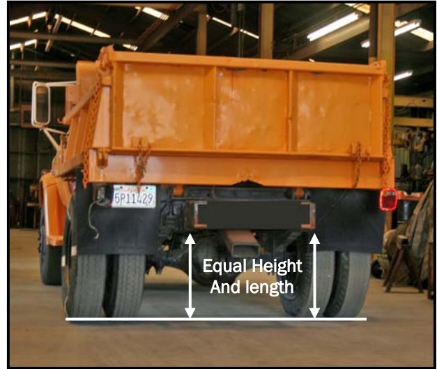
Figure 1. Frame rails are equal Height and length.
