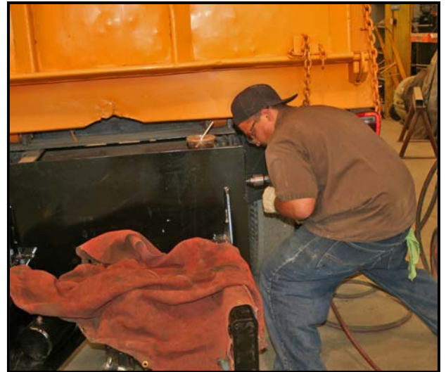
Figure 5. Drill holes through the frame rails.
