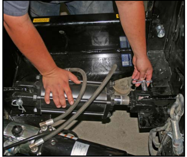
Figure 12. Install the lift cylinder.
