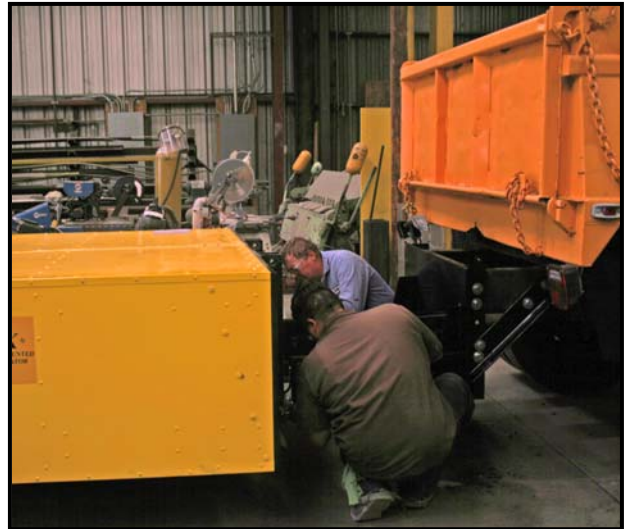
Figure 10. Bolt the TMA to the Support Bracket.
